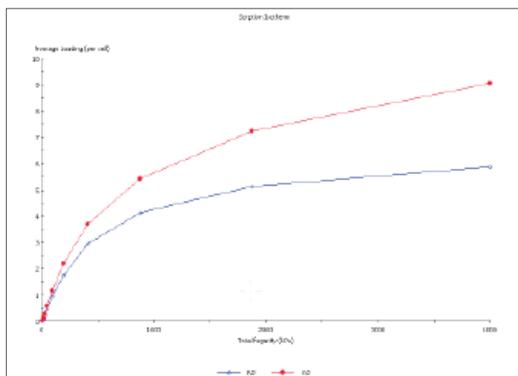
Materials Studio Sorption isotherms for O<sub>2</sub> and N<sub>2</sub> in mordenite at 300 K as computed by Materials Studio Sorption. The ability to handle mixtures of sorbates is critical to modeling processes of separations and diffusion.
