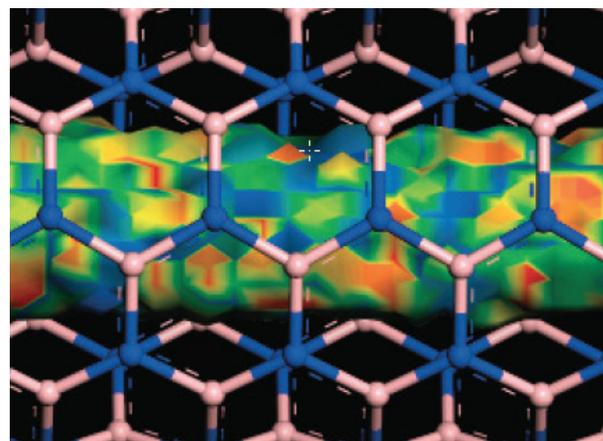
Materials Studio Sorption can be used to study gas storage in nanotubes. The figure represents H<sub>2</sub> sorption in a boron-nitride nanotube. Nitrogen atoms are blue and Boron pink. The surface illustrates an isodensity surface of H<sub>2</sub> mass density within the nanotube. The surface is colored by the potential energy: red indicates lower energy (tighter binding) and blue higher energy.
