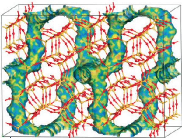
Representation of the sorption of CH<sub>4</sub> in zeolite MFI at 100 kPa and 300°K. The figure shows an isodensity surface of the predicted locations of CH<sub>4</sub> colored coded by the binding energy. Lower energy (more tightly bound) areas are in red and high energy areas are blue. A representation of this type will indicate areas of highest concentration of the sorbates as well as preferred binding sites in the cavities.
